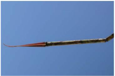
Steel adaptor and long insert prevented bending back of taper, but bent broadhead deviated arrow's path, reducing penetration and breaking this carbon shaft further up. Predictable performance requires total arrow integrity: broadhead, broadhead taper, insert and shaft.
