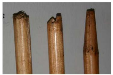
The most common point of wood shaft failure is also at the taper.
